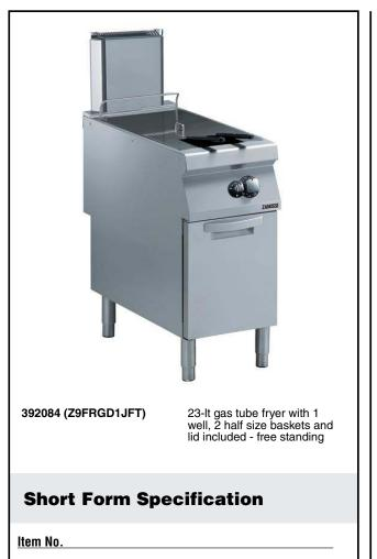
High efficiency 19 kW burners in stainless steel. Gas tubes (heat exchangers) inside well. Suitable for natural gas or LPG. Oil drains through a tap into a container positioned under the well. Height adjustable feet in stainless steel. Exterior panels in stainless steel. Worktop in 20/10, stainless steel. Right angled side edges eliminate gaps and possible dirt traps between units.
